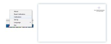
In order for calibration to be successful, hold the cross for about 2 seconds, until it jumps to the next calibration point. After calibrating all 4 points, the board will save the coordinates of the displayed image. Calibration must be performed again each time when the position of image displayed on the board is shifted.
